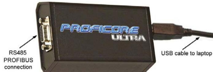
Normally we use a small “tap connector”, which is actually a 100mm stub line to connect ProfiCore to the network. This may sound strange, but actually is very useful as we can see the very small reflection caused by the tap connector and with this make cable length measurements (see example below).
