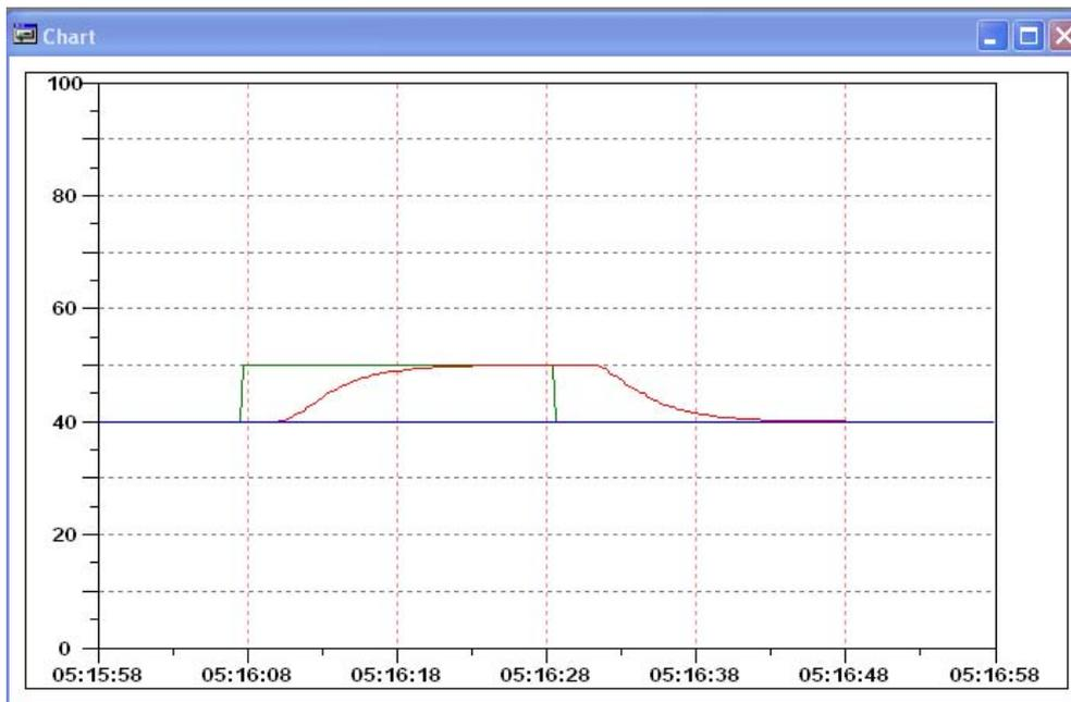
Figure 4 – The open-loop step response of the example plant
