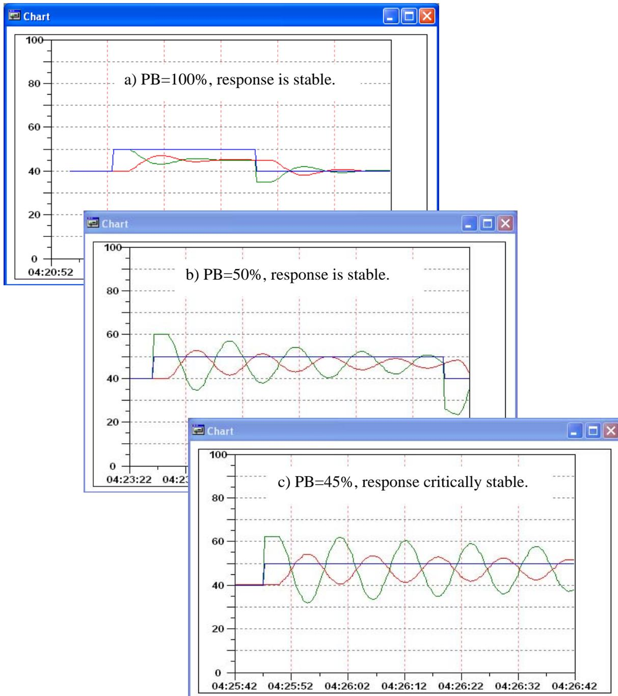
Figure 2 – Typical results from a continuous cycling tuning exercise
