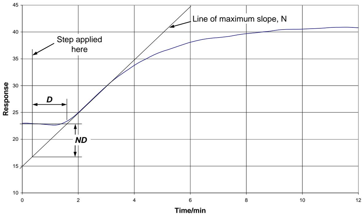
Figure 1 – The Ziegler-Nichols reaction curve method
