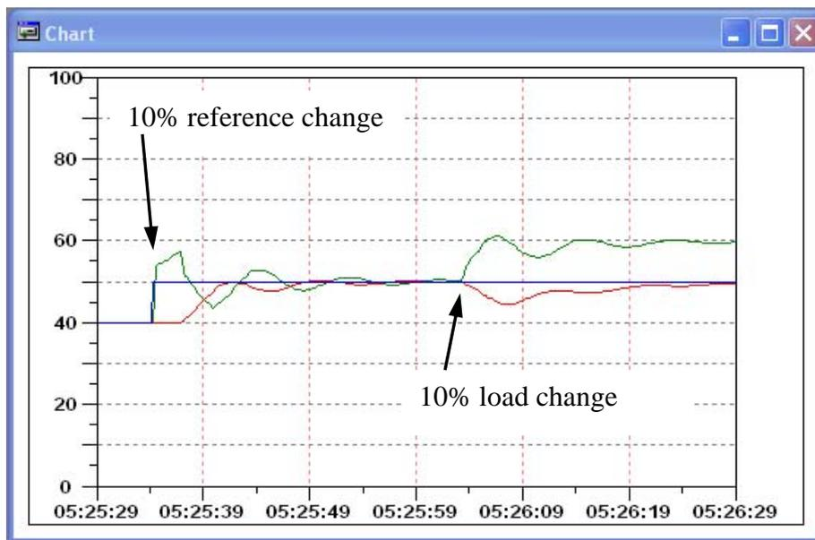
Figure 3 – Response of a PID controller tuned according to Z-N continuous cycling method
