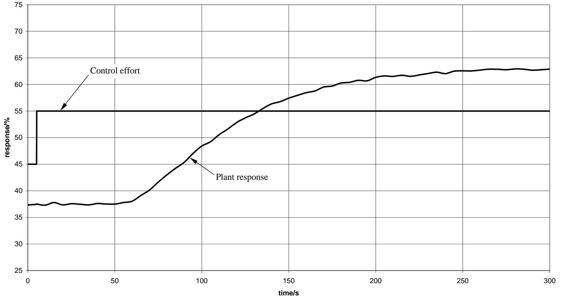
Figure 6 – Reaction curve of a process plant
