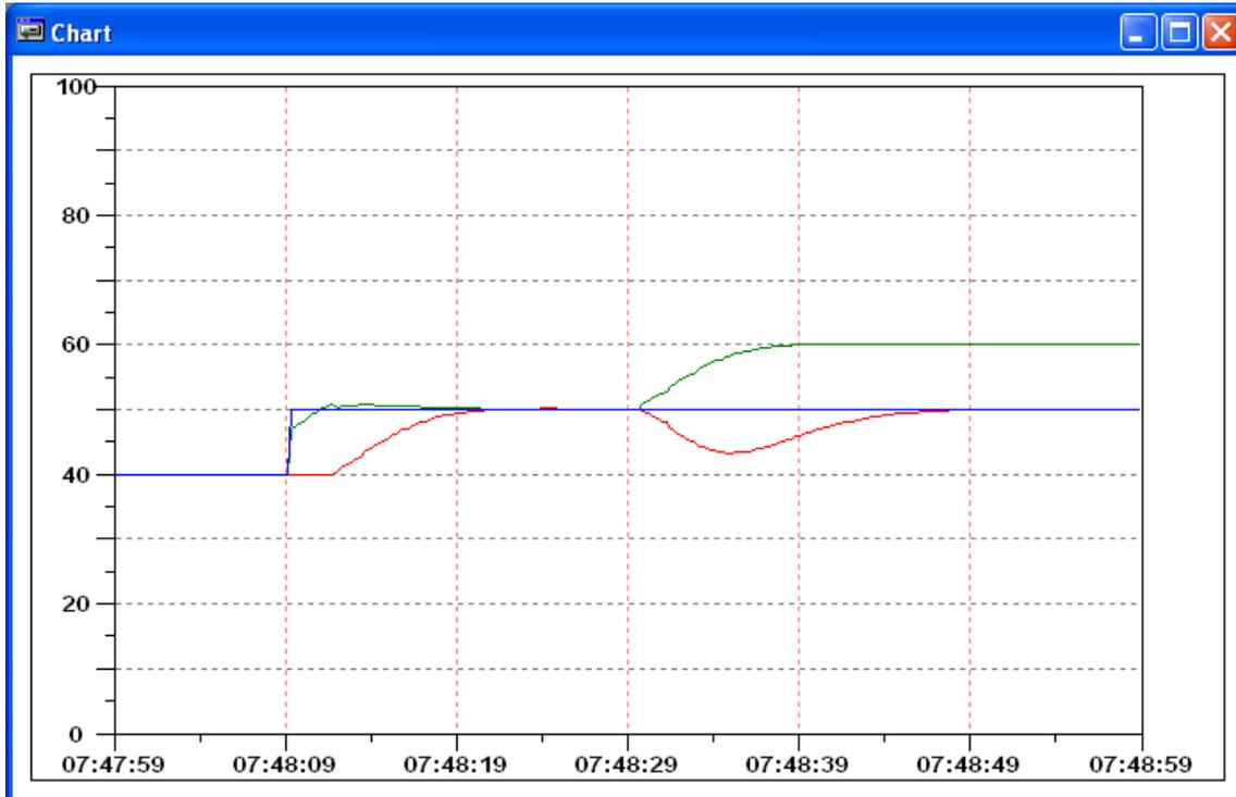
Figure 5 – Response of a PID controller tuned according to Brambilla’s method
